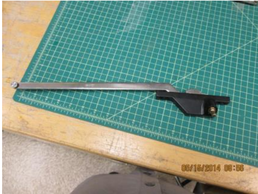
Photo No. 3 Face - Mount Single Arm - SST - Before 300 Hour Salt Spray
