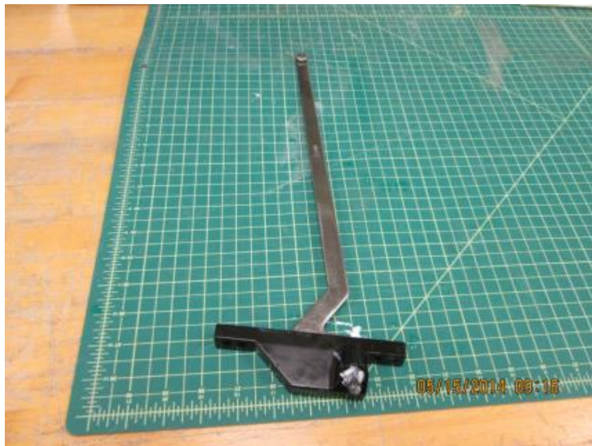
Photo No. 4 Face - Mount Single Arm - SST - After 300 Hour Salt Spray
