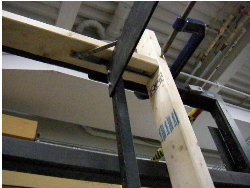
Photo No. 4 10" Hinge Cycling Installation - Top Hinge Detail
