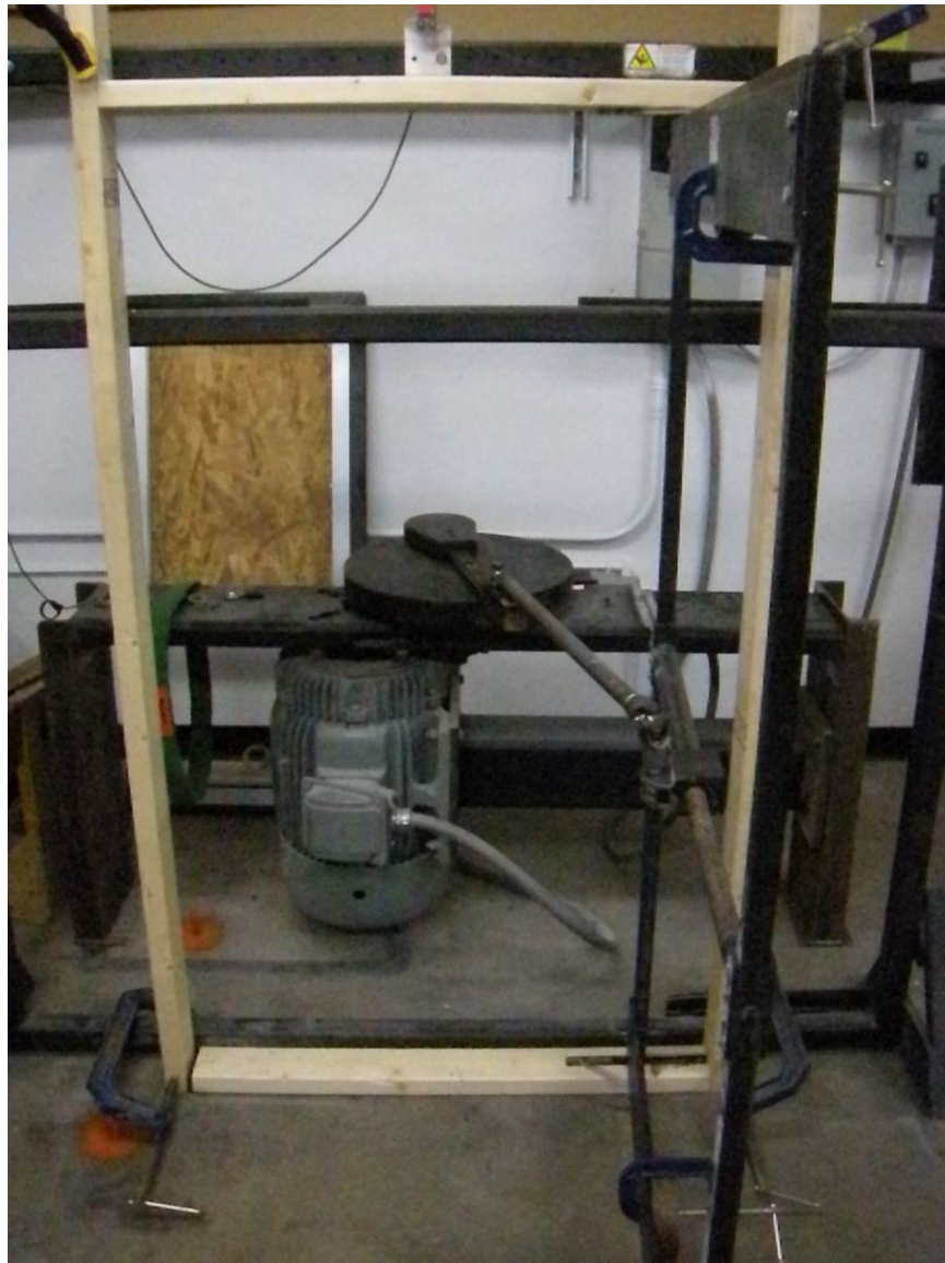
Photo No. 2 10" Hinge Cycling Installation - Open Detail
