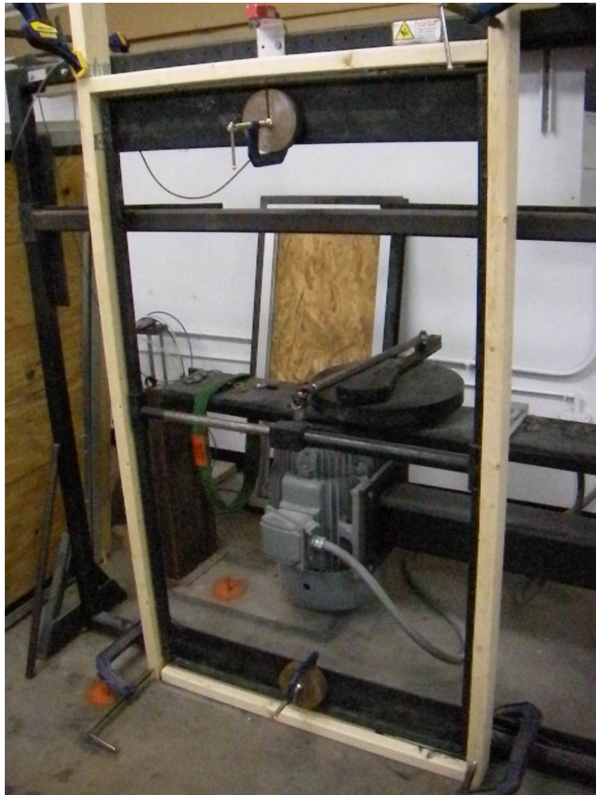
Photo No. 1 10" Hinge Cycling Installation - Closed Detail
